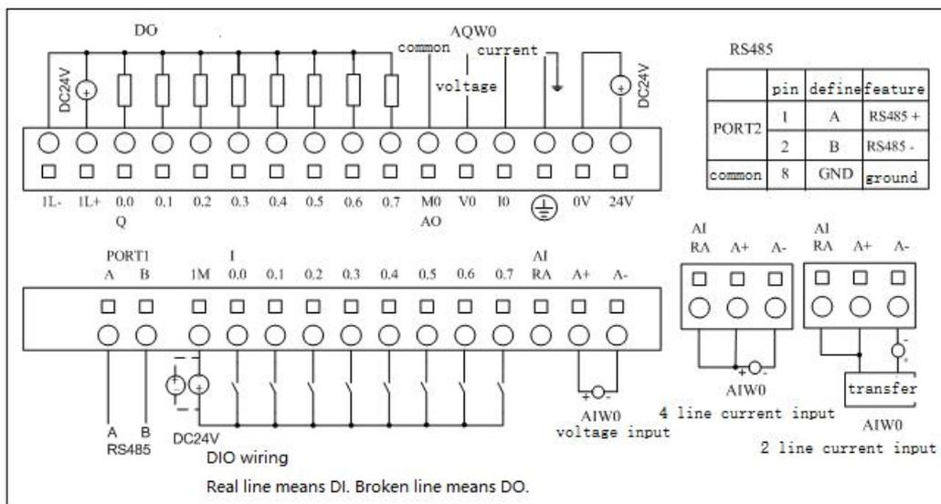
Fig.2-4 K205EA-18DT wiring diagram
