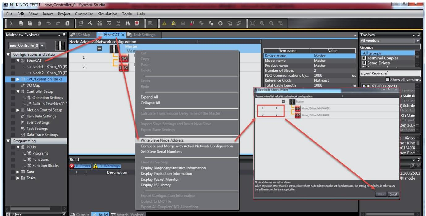
Reboot controller and servo driver to online again. We can see the servos are connected correctly in EtherCAT frame. If connected wrong, it will show X mark instead of triangle.
