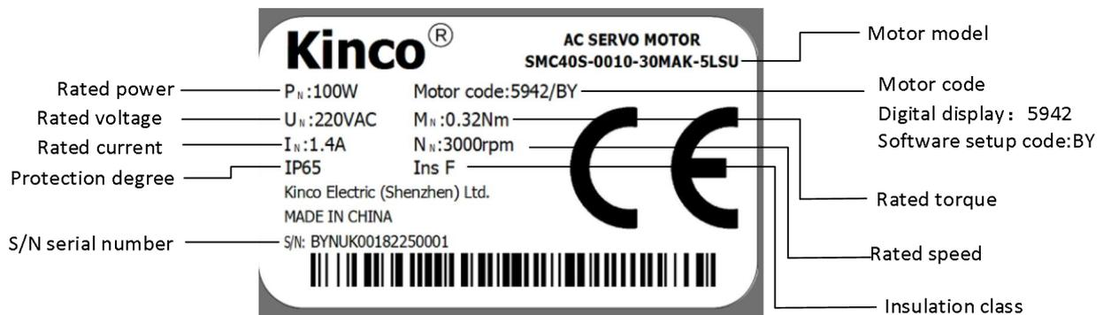
Figure 1-4 Motor nameplate description
