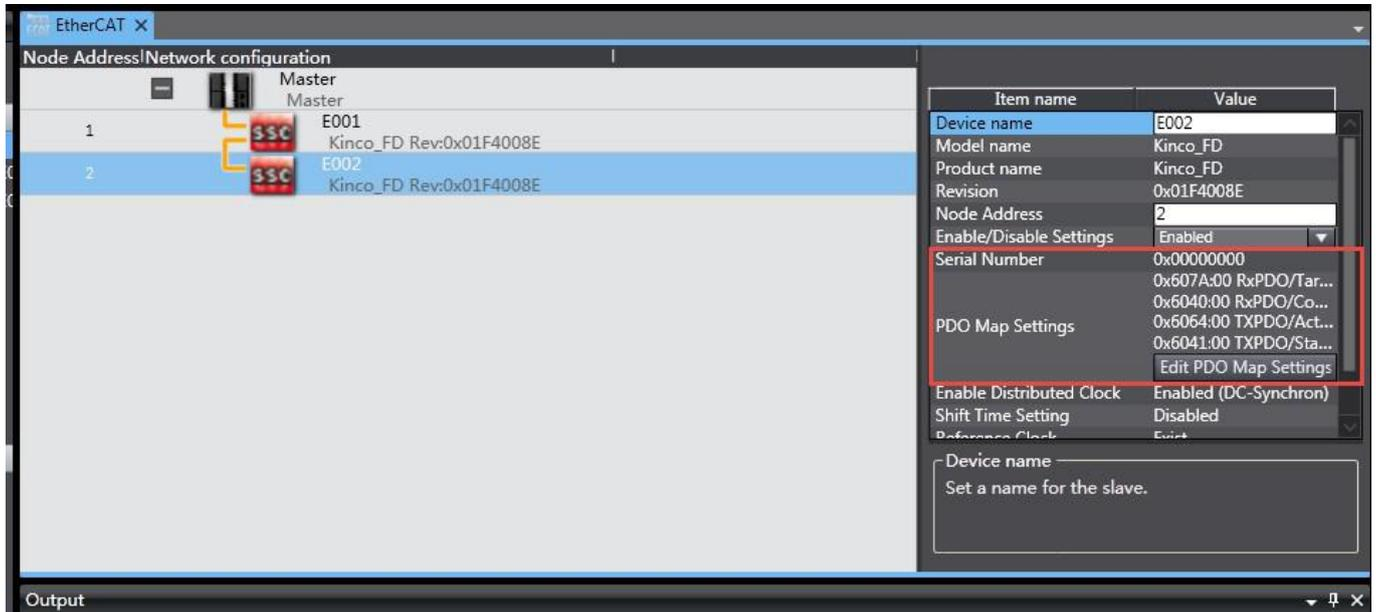
For more control demand, for example to use Ethercat as an ordinary slave station instead of motion control, it needs to add and configure more PDO. Click Edit PDO Map Settings to choose output RPDO or input TPDO channel and then add PDOs. Last, click Apply and Ok to be available.
