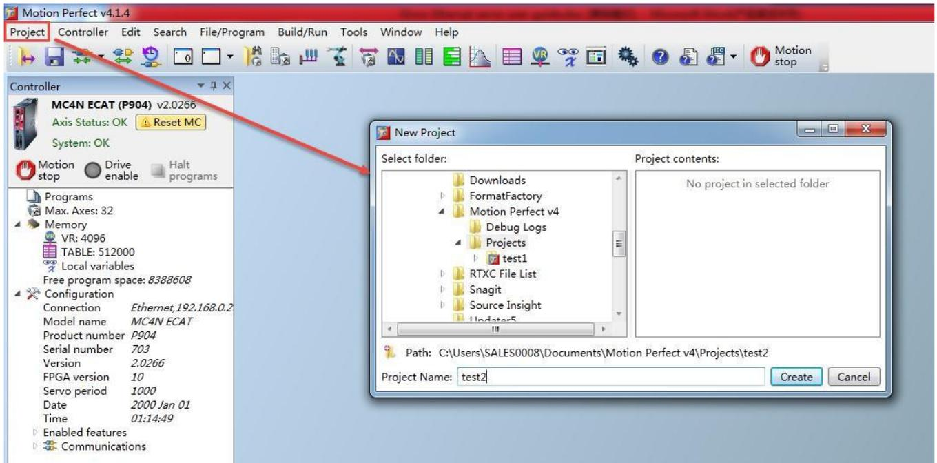
After created the project, software will change to sync mode automatically. First, import slave information file, while Trio controller doesn't support import XML file directly, the slave information file needs to be written already in software when the software is released. Before unsupported, use below guide to import slave information file EC\_EXTEND.TXT. This file can be downloaded in Kinco website.
