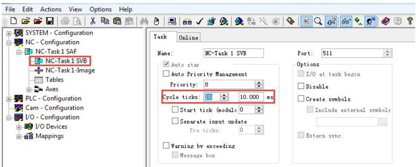
Set the unit of NC. In Axis 1\_Enc, Scaling Factor which means the distance for each pulse feedback from encoder should be set. For example, Kinco servo motor has 10000 pulses for a round and if the moving distance is 1mm, then the Scaling Factor should be  $1/10000=0.0001\text{mm/Inc}$ . If the real position increase 10mm, then target position in servo should increase 100000INC also. Normally, it needs to set some relative speed parameters for NC control in Axis, else the servo may show alarm.
